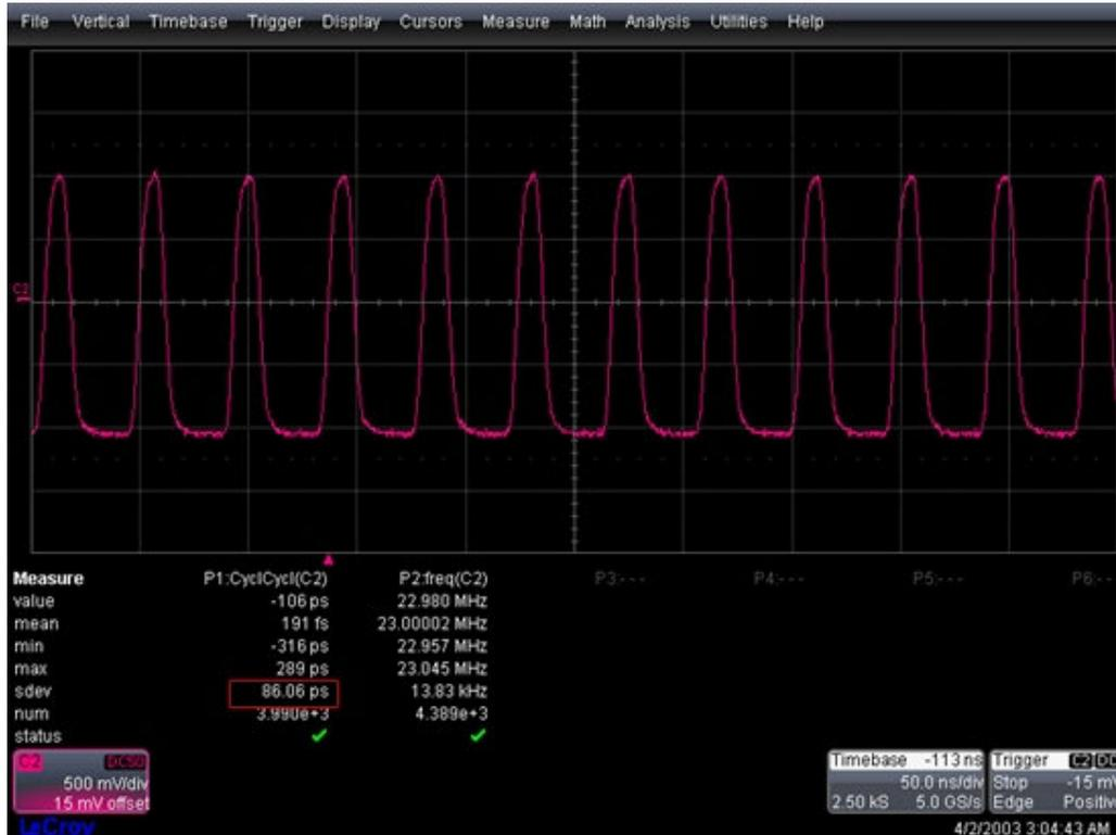
P4 EasyPulse waveform with low jitter
